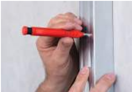
TLM2 for markings up 1.7 inches depth.
